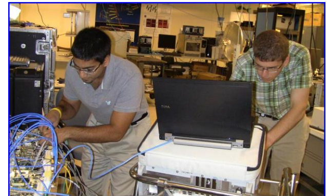
Shahil Kantesaria and Nathan Olivarez assemble a software-defined radar (2011).
