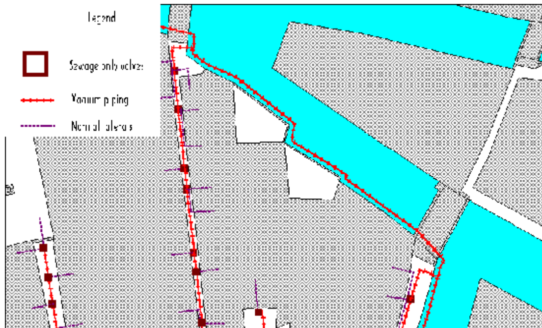
Figure 3: Option two proposal of vacuum sewerage implementation.
