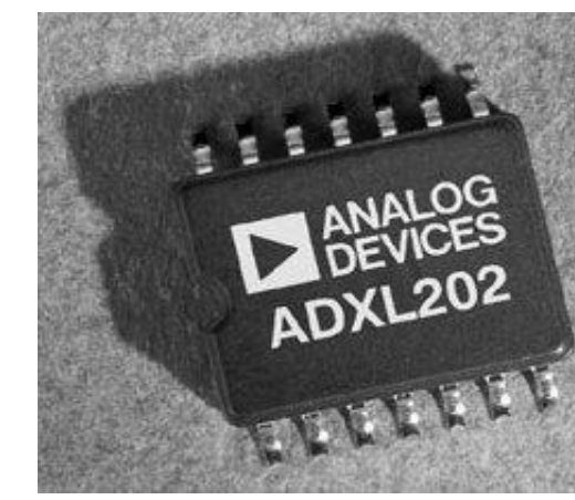
Analog Devices' ADXL202 micro accelerometer
