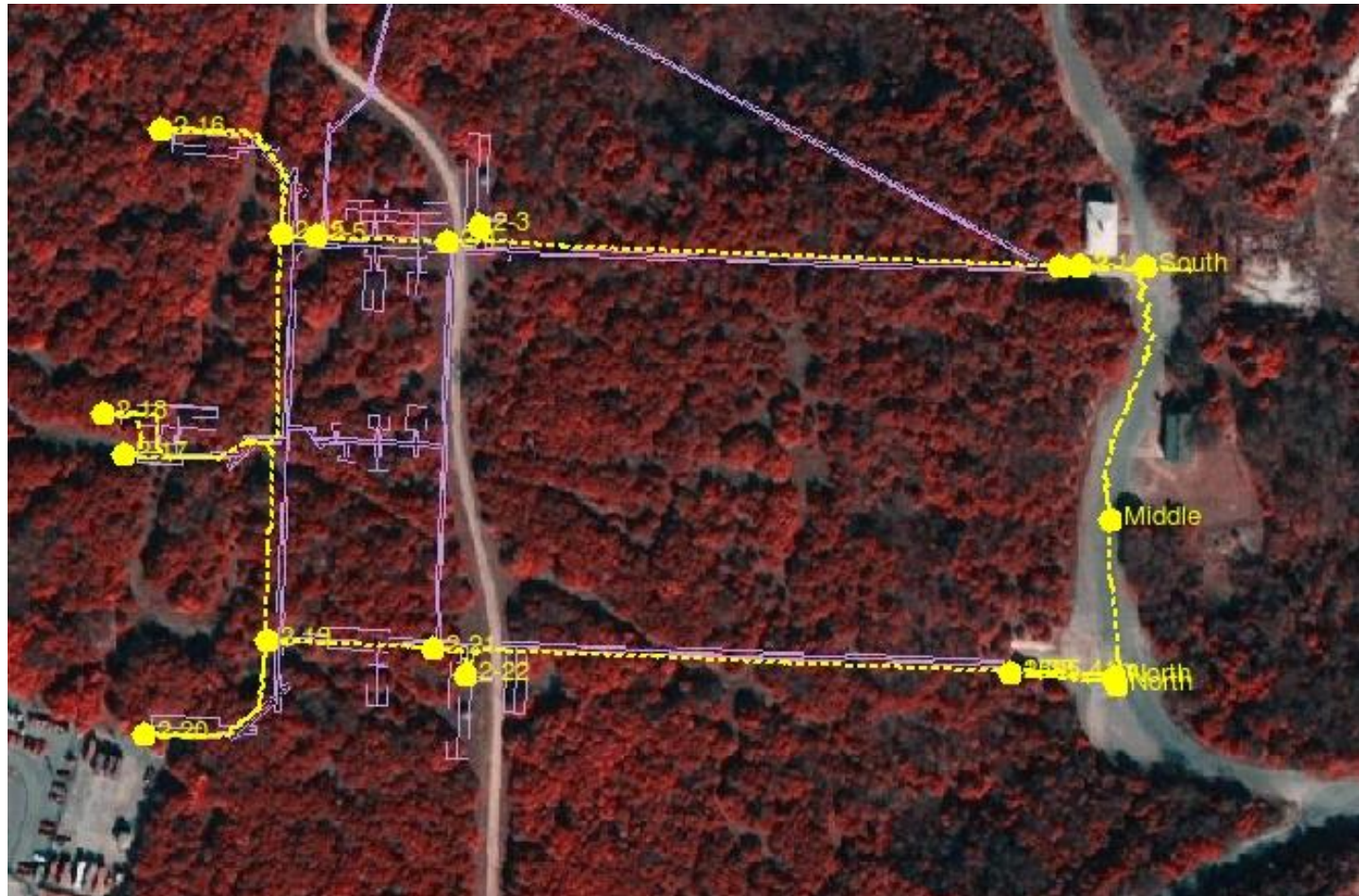
Tracks in Fort Hood Tunnel Complex with HG-1930 and Track Correction Algorithms Less Than 1% x, y, z, error over 1 km distance
