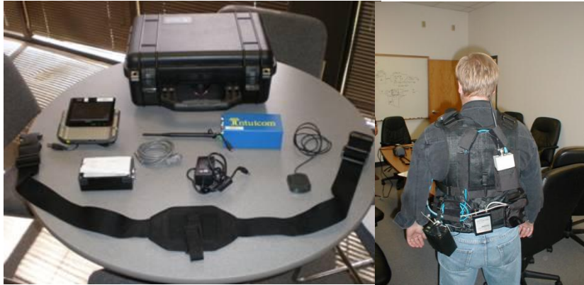
Spiral 0: DRM-5, OQO Computer, external GPS, Harris/CHI SA software, UHF data radio
