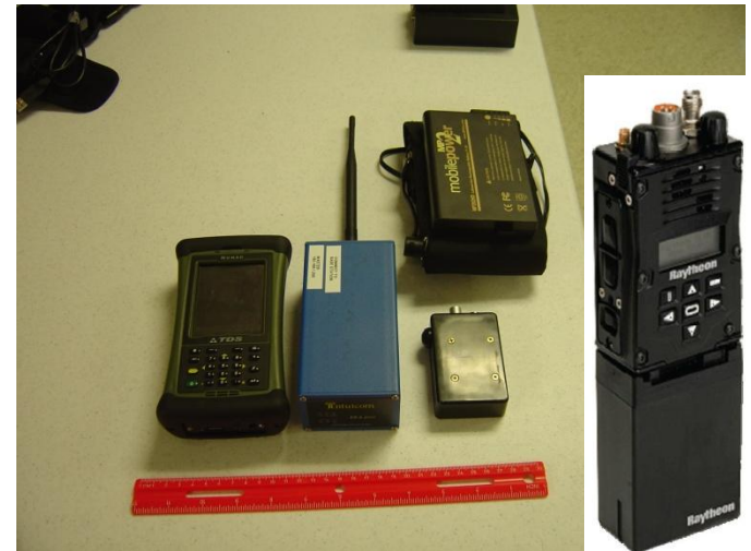
Spiral 1: DRM-4000/5000, Nomad hardened PDA, DTRA or commercial UHF data radio, improved Harris/CHI SA and navigation software, power supply
