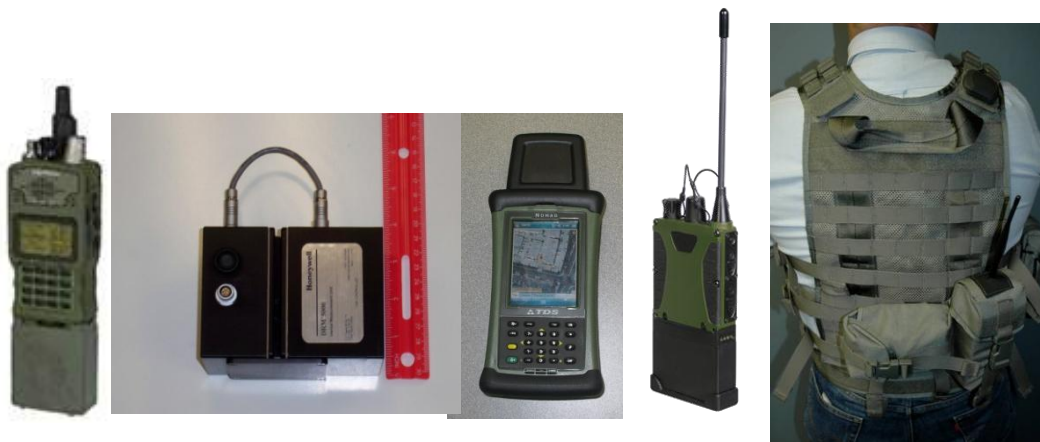
Spiral 2: DRM-5000 plus HG-1930 IMU, Nomad hardened PDA, military voice/data radios, improved Harris/CHI SA software and track correction algorithms
