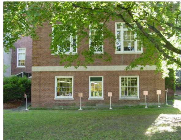
Fig. 3 The exterior view of the indoor test conducted in WPI's Kaven Hall. Base antennas surround building wing on three sides.
