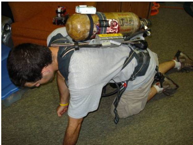
Fig. 9 Crawling tests to provide different antenna orientation
