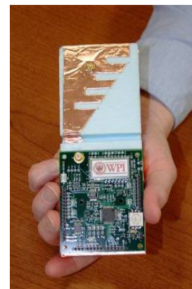
Figure 8: Locator concept drawing and photo of prototype PIFA antenna with circuit board
