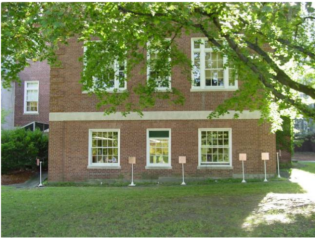
Figure 16: The exterior view of the indoor test. Base antennas surround the building wing on three sides.
