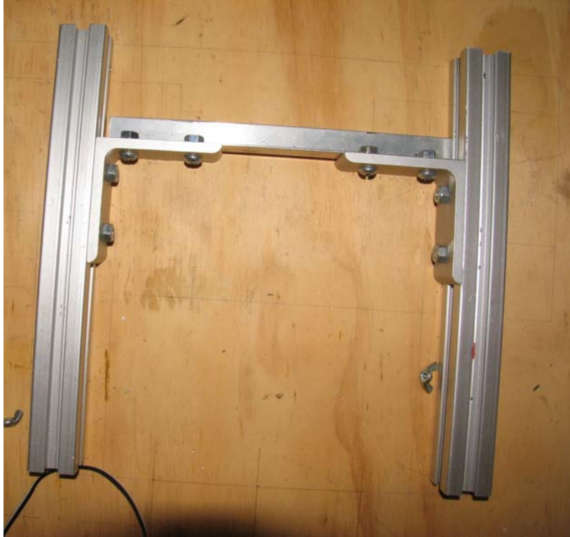
Figure 5 - H-frame track for leaf springs mount.
