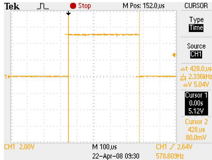
Figure 33: Bit Length of One Bit of PIC Output
