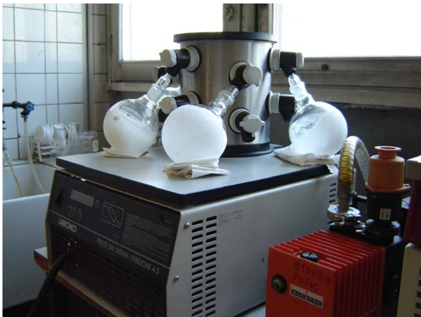
Figure 25: Labcono Freeze Drying System
