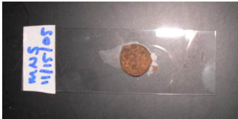
Figure 9: Slide with disc of crust ready to be viewed with the epifluorescence microscope
