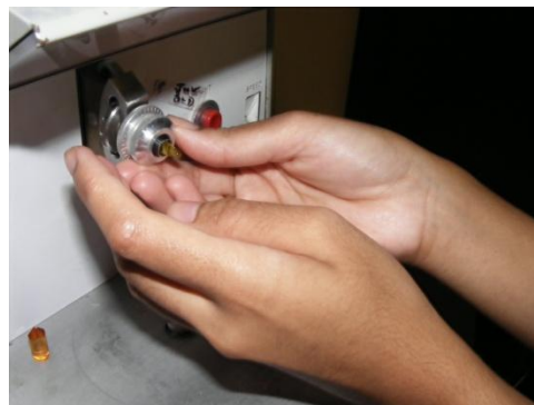
Figure 5: Assembly of resin-embedded specimens onto Sorvall Porter-Blum microtome machine
