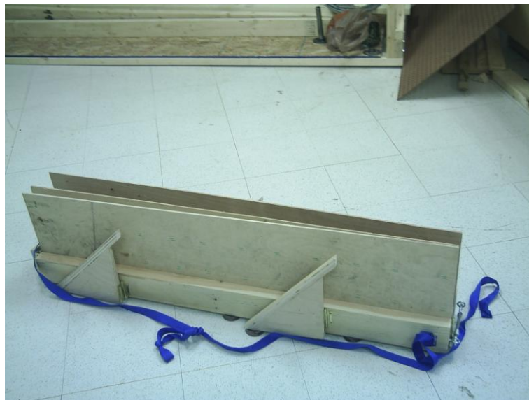
Figure 27: Backstop Panels in Stored Position
