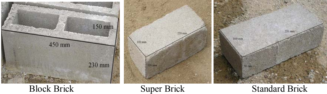
Figure 4.7: Comparison of block, super, and standard bricks from Makalani Bricks.
