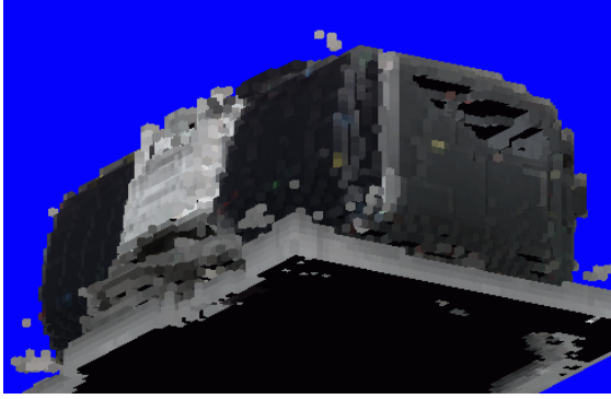
Figure 5.7: Histogram fails to reconstruct right side
