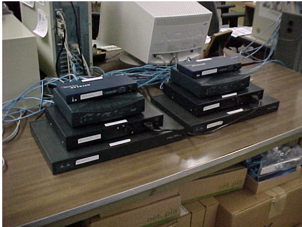
Figure 7.2: Pictures of routers and switches that were used during the testing of the Switched Fault Tolerance System.
