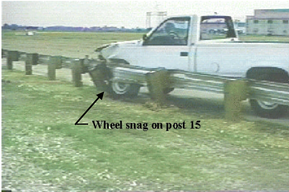
Figure 1. Full scale test showing wheel snagging. (6)
