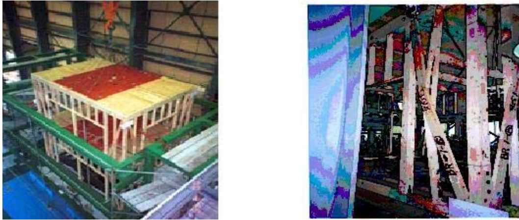
Figure 3.10 Two-story wooden structure (left) and observed damage (right)
