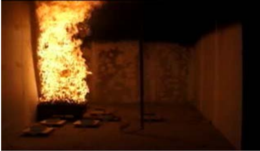
Figure D 14 A Photo of 1 MW Fire in Propane Characterization Experiment.
