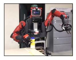
tional Neural Networks (Mask-RCNN) models to create a final model for determining both object location and grasp angle. This allows the Baxter Robot to autonomously detect and reach towards the object. Using learning by demonstration, the robot can learn how to grasp and manipulate said objects.
