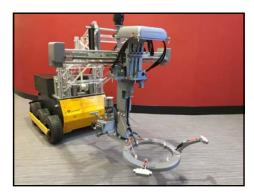
tocopter drone will work in tandem to locate, mark and eliminate anti-personnel landmines in a user-defined location.
