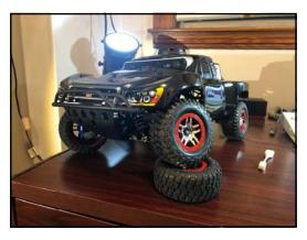
ment unit, and other sensors to observe the environment. Completed research explored pose estimation based on combining dead reckoning, inertial measurement unit readings, and visual odometry in an Extended Kalman Filter. The result of this project included the RC car and a build guide on replicating the process for future students.
