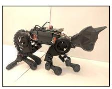
gree-of-freedom (DoF) legs, a continuum tail, and 3D printed body and construction. This will all be powered by custom servo motor controllers and 9DoF IMU sensors, all connected to a custom embedded SPI daisy chain protocol running on a custom microprocessor. The higher level controller will
