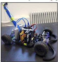
track. Prior to conducting autonomous testing, a custom made scale car was designed and manufactured. Comprised mainly of 3D printed parts, the car had rear-wheel drive with passive independent front and rear suspensions. To enhance the car design, tachometers, strain gages, temperature sensors, and an inertial measurement unit were integrated to
