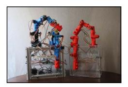
vice. The addition of a simulation environment to visualize the forward/inverse kinematics as well as fully functioning hand controls for TRINA allows for a more user friendly working system. This article discusses the process of the fabrication and implementation of the circuitry, hardware, and programming for the first iteration of the active version of the Telenursing RoboPuppet.
