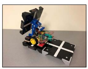
task. Our system uses a network of intelligent scaffolding blocks to direct a simple manipulator robot to construct two dimensional structures from dedicated building blocks. This project incorporates a processing work, heterogene-
