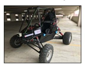
MQP team designed and developed a Level 3 autonomous vehicle prototype using an SAE baja vehicle outfitted with actuators and exteroceptive sensors. At the end of the team's work, the vehicle had a driveby-wire system, could localize itself
