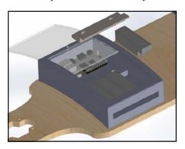
equipped with two motors controlled by a handheld RC controller and is capable of achieving speeds as high as 20 mph. The deck can be disassembled and reassembled by hand to swap out major mechanical components of the board. The board's electrical
