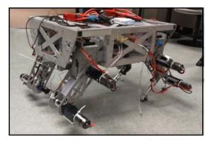
to ensure that the robot quadrupedal chassis build by a previous MQP could move stability and intelligently so that it can be useful for future projects. Three main motion gaits were studied, a crawl gait, a walking gait, and a turning gait. The project implemented stable motion for the three gaits mentioned. In addition, the team also made significant system design improvements in the structure, electrical circuit, and code.
