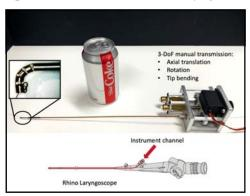
ness is limited by the restricted range of motions attainable by state of-the-art surgical instruments. In this project, we propose a new ultra-thin dexterous manipulator made of super-elastic Nitinol intended to amplify a surgeon's manipulation capability during endo-
