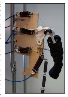
Muscles and a biomimetic UCL. The effectiveness of the brace was validated by interfacing it with the robotic arm and measuring the forces on the artificial UCL throughout the pitching phases.
