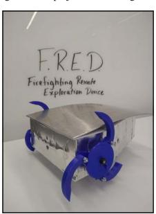
fighters with additional information about a fire environment to help them make more informed decisions when fighting a fire. We have built a prototype robot that is compact and quick to deploy, with a heat, water, and impactresistant chassis designed to function in unpredictable firegrounds. The remotecontrolled robot returns a real-time video feed and a heat map of a designated area in a building.
