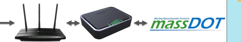
The zed-f9p is RTK equipped, meaning it can achieve up to 3cm levels of accuracy by triangulating with a known ground station. The Pi enables this accuracy by constantly receiving data from the Massachusetts Department of Transportation over an on-board 4G cellular network. These data are then piped into the GPS using ROS.
