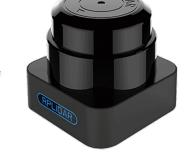
The Jetson communicates directly with an outdoor rated RPLIDAR S1 2D LiDAR system to avoid obstacles in the local environment.
