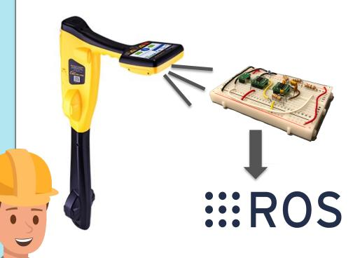
The robot uses a vLoc3 RTK-Pro Utility Locator from Vivax Metrotech to detect electromagnetic fields emitted by underground power cables.
