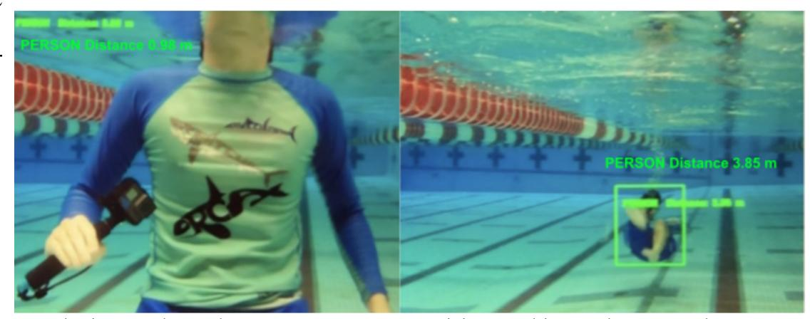
The image above demonstrates our stereo vision working underwater. The program is using an object detection model to track the swimmer and form a boundary box. This boundary box is then used to determine which disparity values are relevant and those values are then used to calculate the swimmers distance. The system is fairly accurate, determining the swimmer is at 0.98 m when he is actually at 1 m and 3.85 m when at 4 m.
