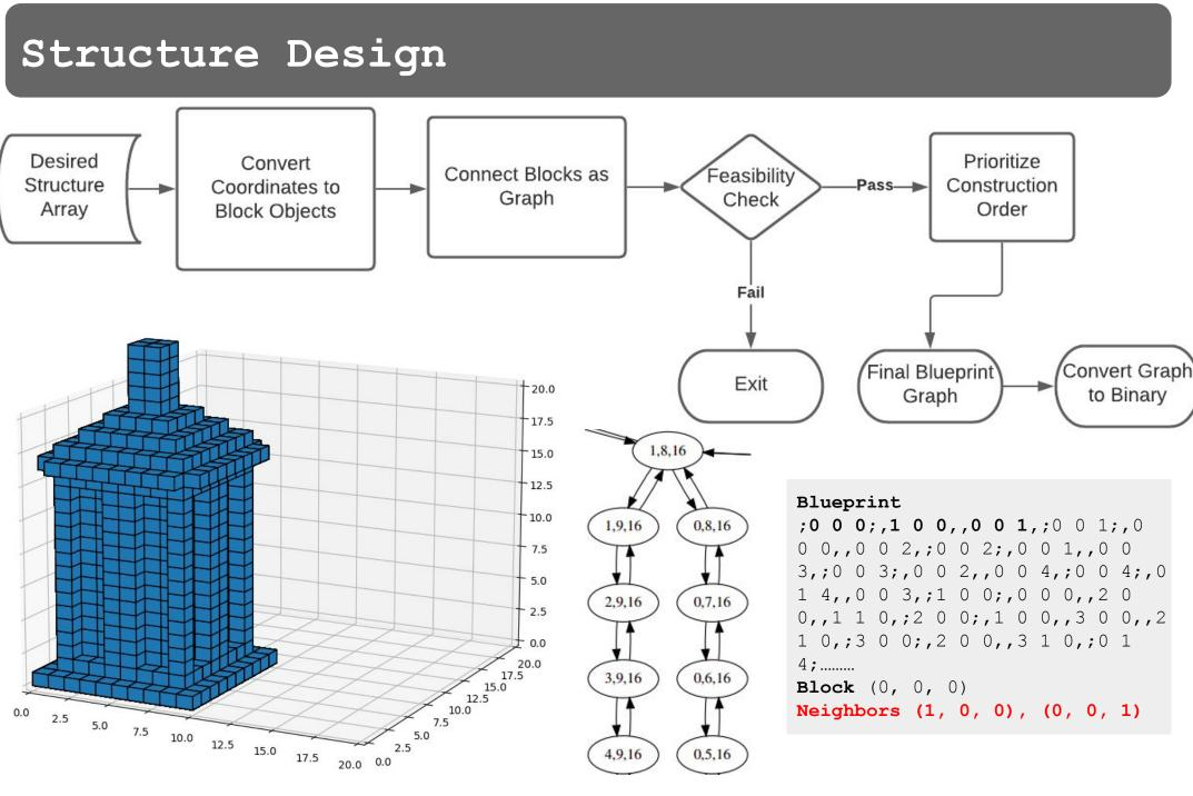
Proposed designs are first ran in simulation. The system is limited by certain rules governing how far blocks can overhang and how much weight they can support. If a structure is analyzed and found to be feasible, each block has their list of neighbors prioritized in a desired building order based on these constraints and the final blueprint graph is produced. This graph is converted to binary for transmission by the blocks.
