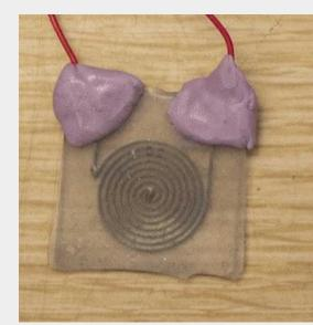
The motorized thumb is powered by two liquid metal sensors. When pressure is applied to sensor 1 the thumb moves forwards, when pressure is applied to sensor 2 the thumb moves backwards. The thumb is powered by a continuous rotation servo that is able to fully close the finger in 0.046s. There is also a solenoid zip tie
