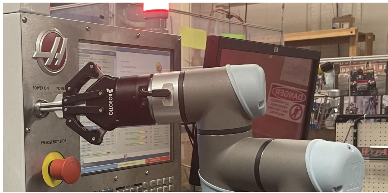
Robot interfacing with control panel Autonomously resolvable alarms
