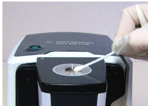
Figure 8. Cleaning the 5 bounce ZnSe ATR sampling window.
