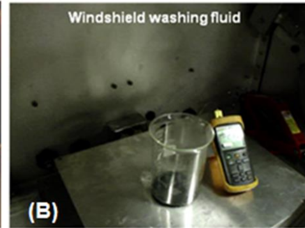
Reactivity of \text{NaAlH}_4 as loose powder (A) and as powder compact (B) when it comes in contact with windshield washing fluid.
