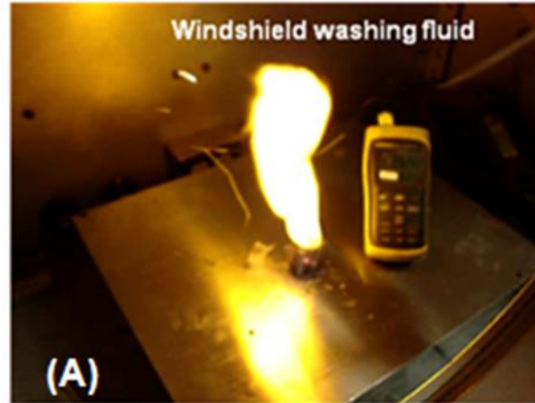
Reactivity of \text{NaAlH}_4 as loose powder (A) and as powder compact (B) when it comes in contact with windshield washing fluid.
