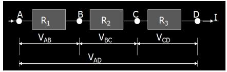
• The overall resistance or **equivalent resistance** (R) is given by:
