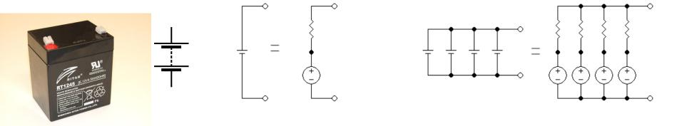
Each cell is a voltage source with a source resistance.
