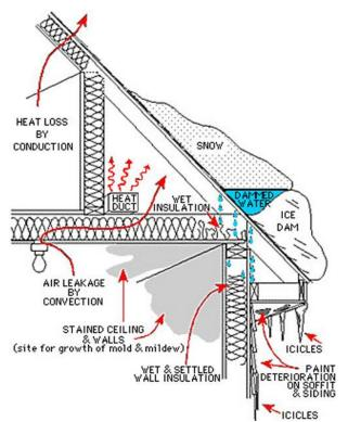
ventilation of the cold roof. This type of roof is completely closed and allows for no air flow. Most roofs aren't as inefficient as one would expect and usually only account for 10% of heat losses (Formisano). The image below (figure 4) depicts some of the potential issues a ventilated space in the attic can create; it will be a potential site for many other issues during the life of the
