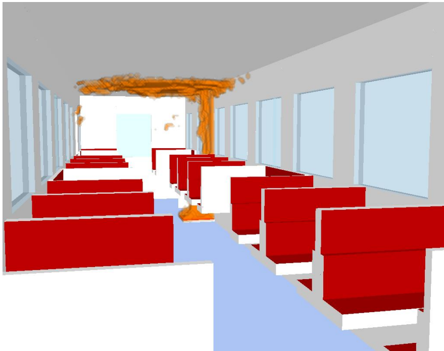
Figure 41. Example FDS Output Showing Predicted Flame Spread
