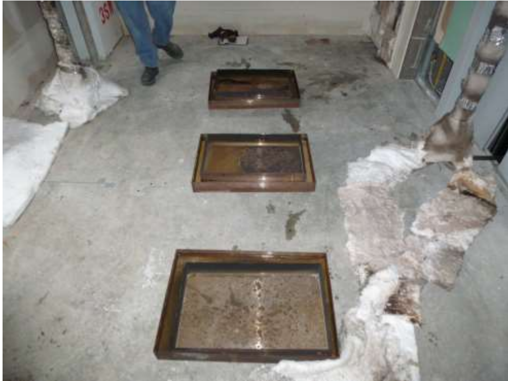
Figure 7.38. Setup of fuel pans and thermocouple trees in the EL
