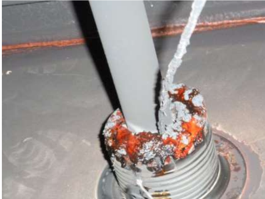
Figure 8.36. Horizontal pipe firestop in corridor after ES fire test
