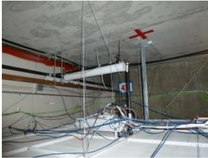
Figure 3.32. Sand weight on Floor 4 sprinkler pipe in the western room area
