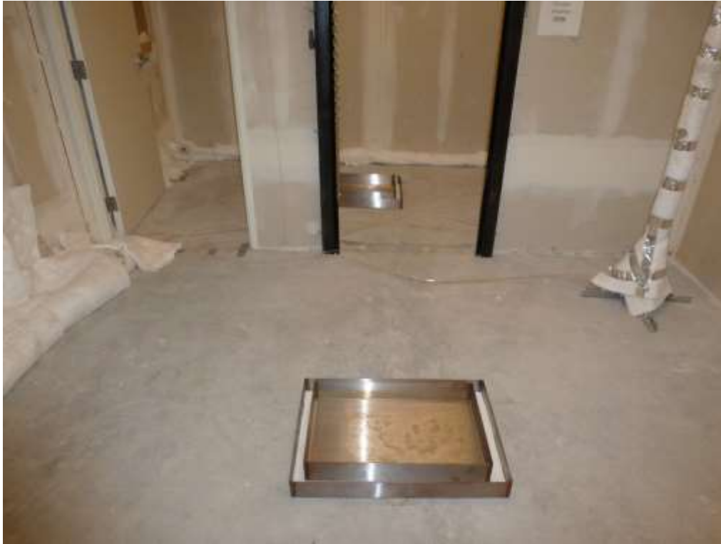
Figure 7.24. Fuel pan and thermocouple tree setup for LBR-1 fire test
