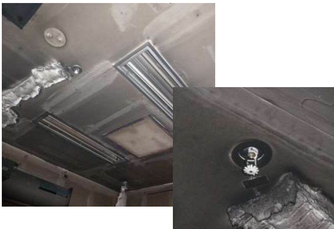
Figure 8.14. LBR sprinkler activation during LBR-1 fire test
