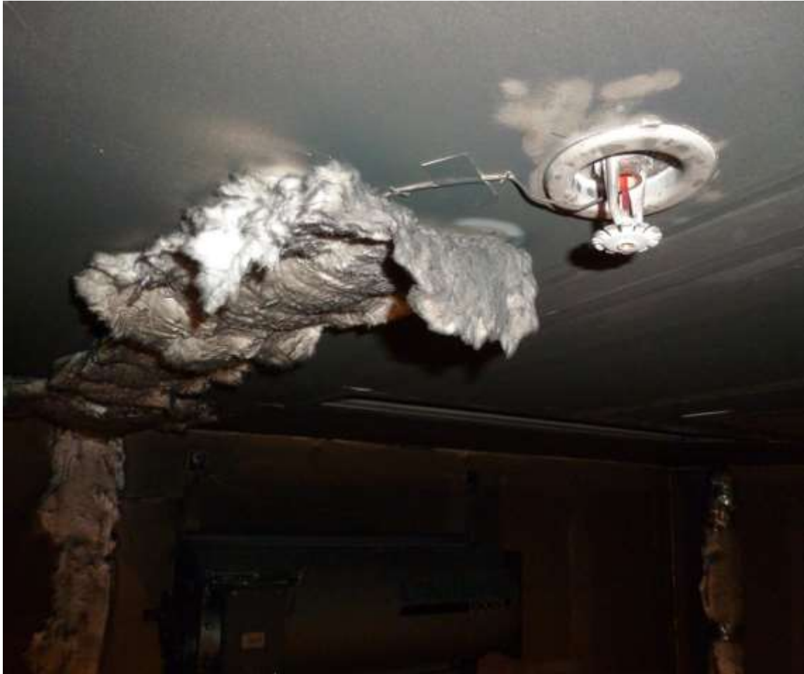
Figure 8.23. LBR sprinkler head after SBR fire test
