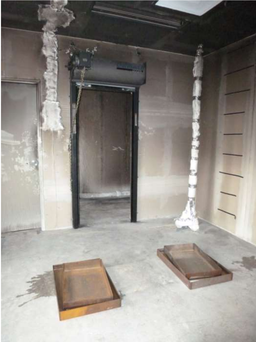
Figure 7.32. Fuel pans and thermocouple tree setup in the LBR
