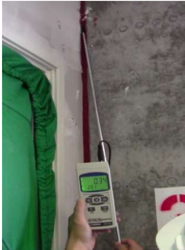
Figure 4.8. Air leak check using an anemometer
