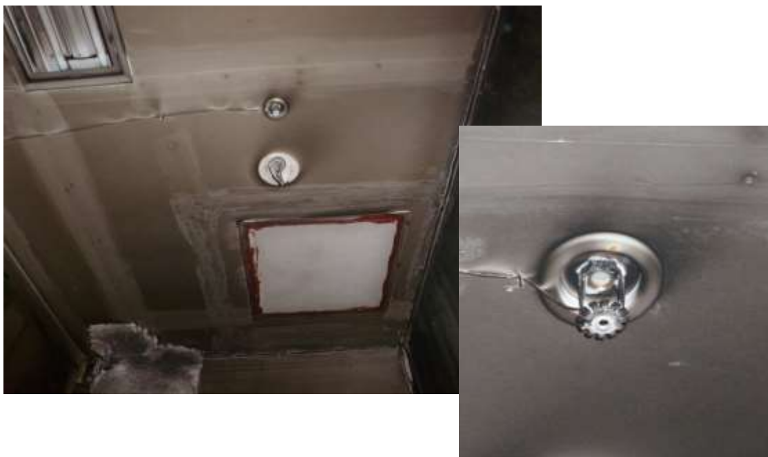
Figure 8.13. SBR sprinkler activation during LBR-1 fire test
