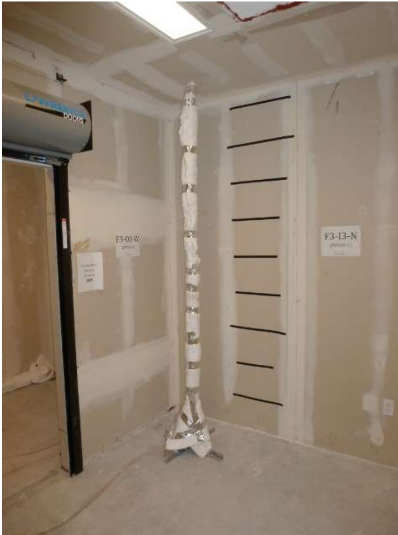
Figure 7.2. TC tree protected with ceramic fiber blanket
