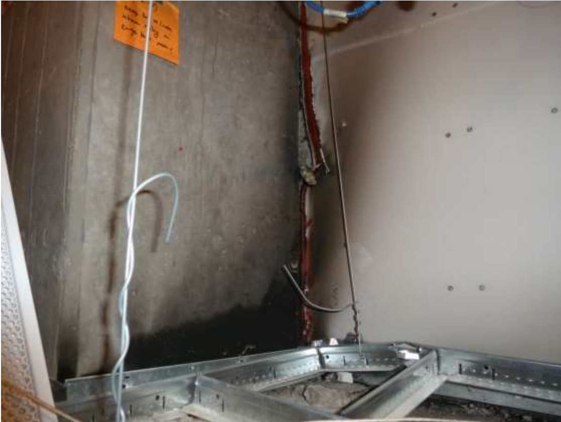
Figure 8.20. Northeast corner in space above SBR ceiling after SBR fire test
