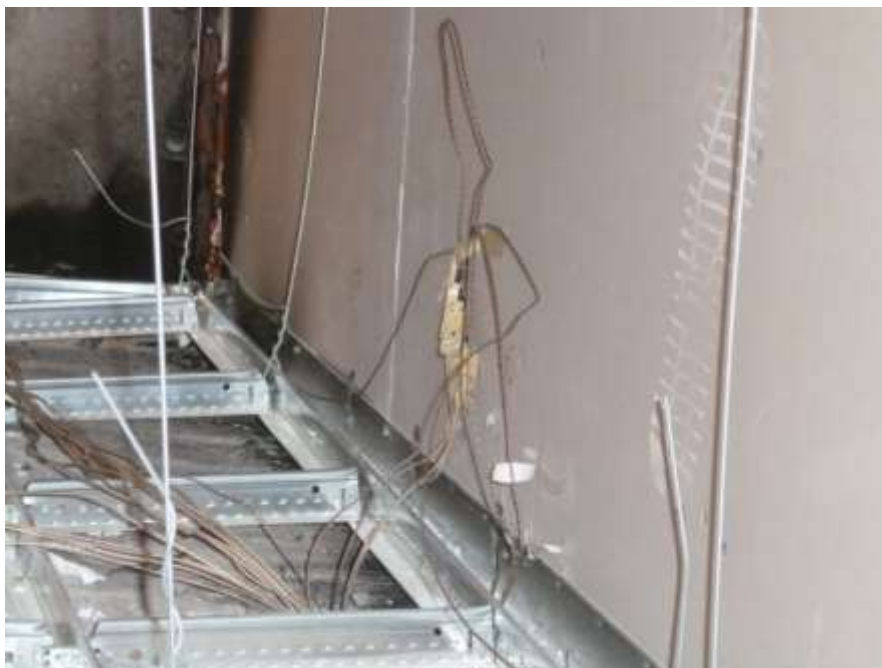
Figure 8.8. Space above LBR ceiling after LBR-1 fire test
