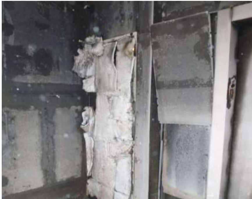
Figure 8.52. South wall of elevator shaft after EL-2 fire test
