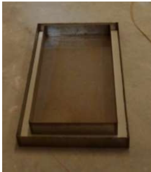
Figure 7.22. Actual heptane pans used for the fire tests
