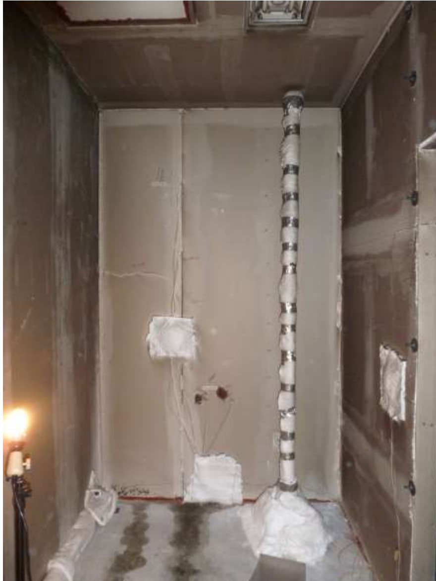
Figure 8.10. South wall of the SBR after the LBR-1 fire test
