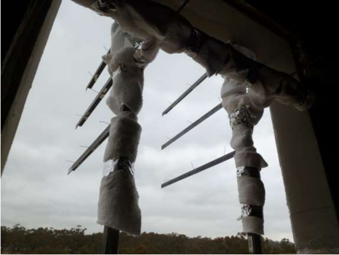
Figure 7.33. Thermocouple trees installed on the LBR window
