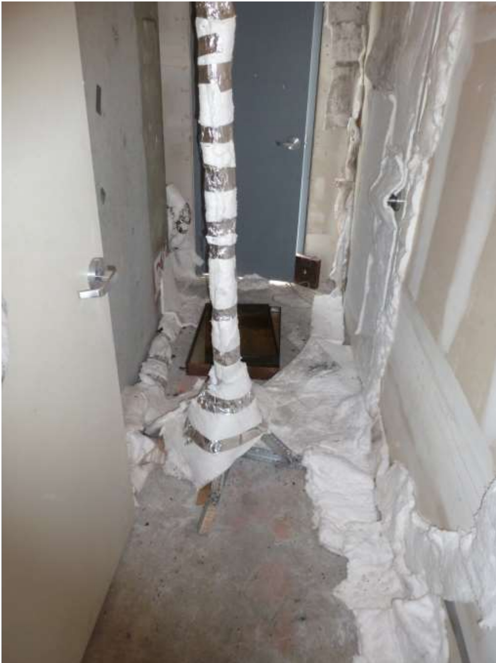
Figure 7.36. Fuel pan and thermocouple tree setup in the corridor area
