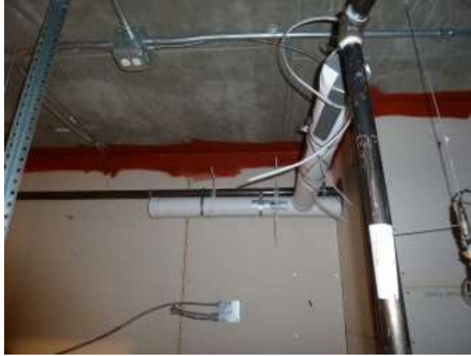
Figure 3.12. Sand weight on Floor 1 sprinkler pipe in the room area
