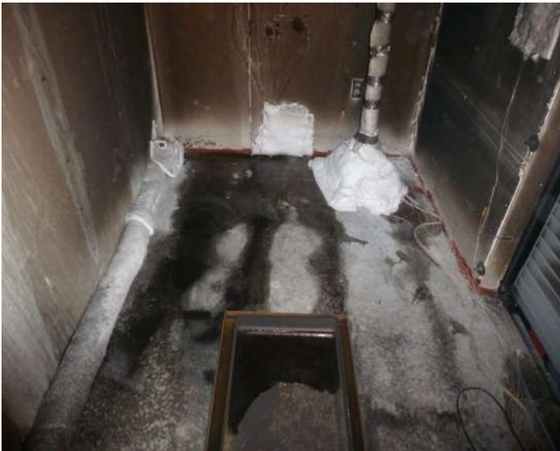
Figure 8.18. SBR after SBR fire test
