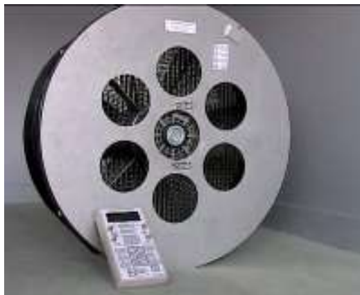
Figure 4.4. Low-flow plate attached on back of fan
