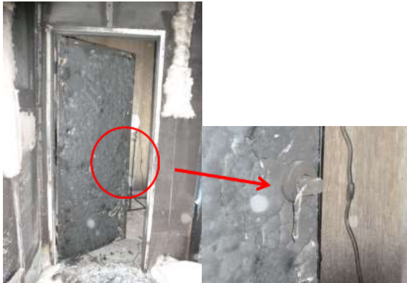
Figure 8.28. Partition wall door 1 after LBR-2 fire test
