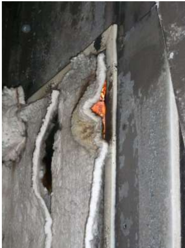
Figure 8.53. Door 4 after EL-2 fire test
