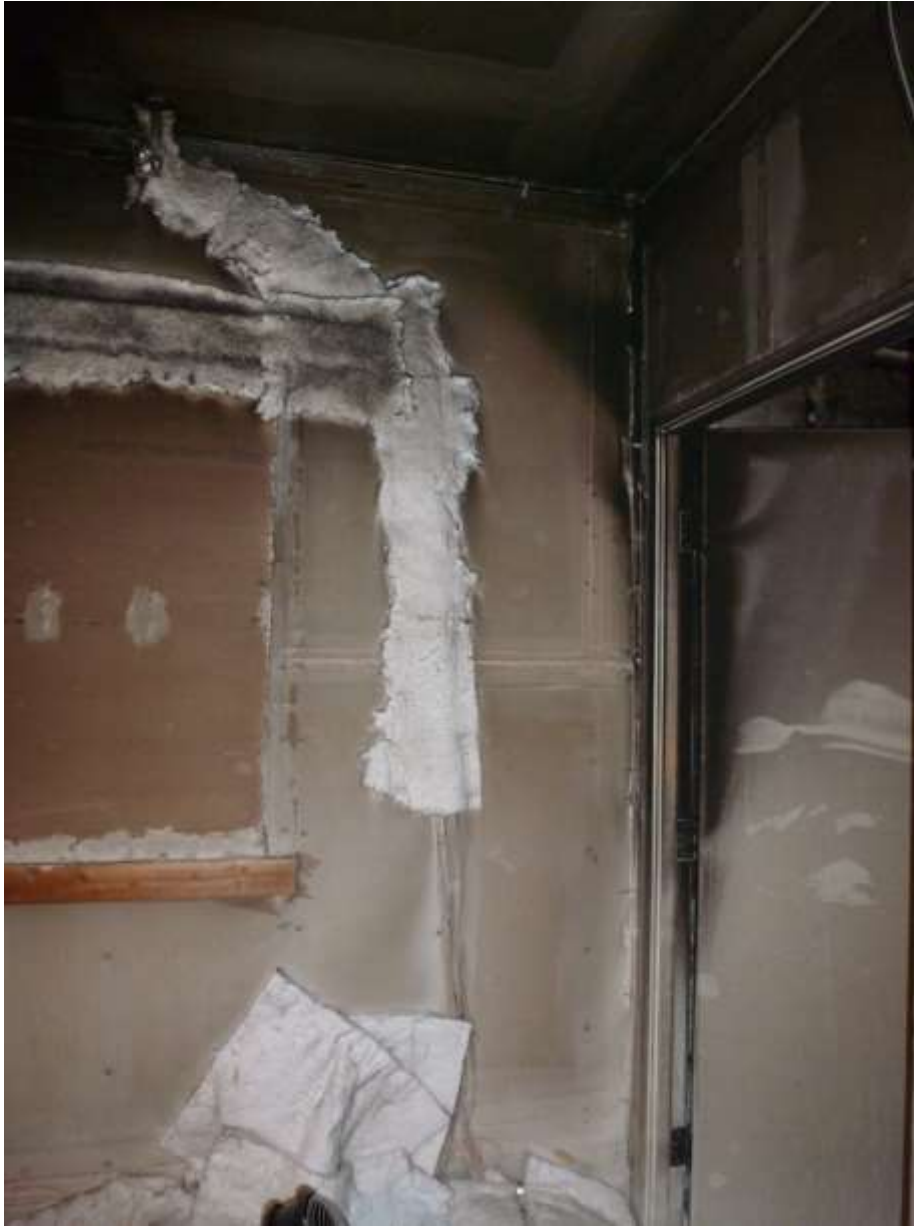
Figure 8.21. Partition wall gap after SBR fire test
