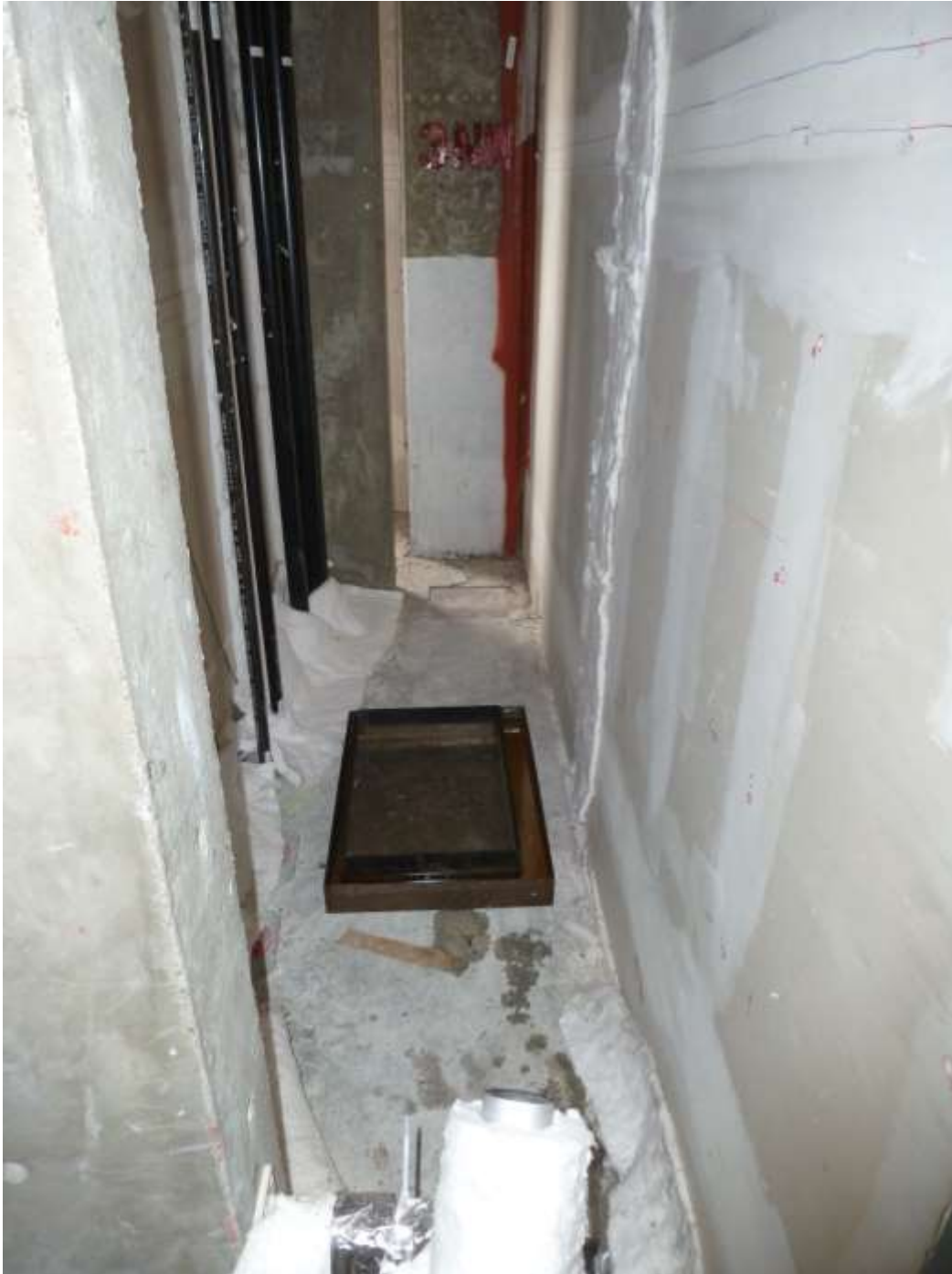
Figure 7.35. Fuel pan setup in the space north of the elevator shaft
