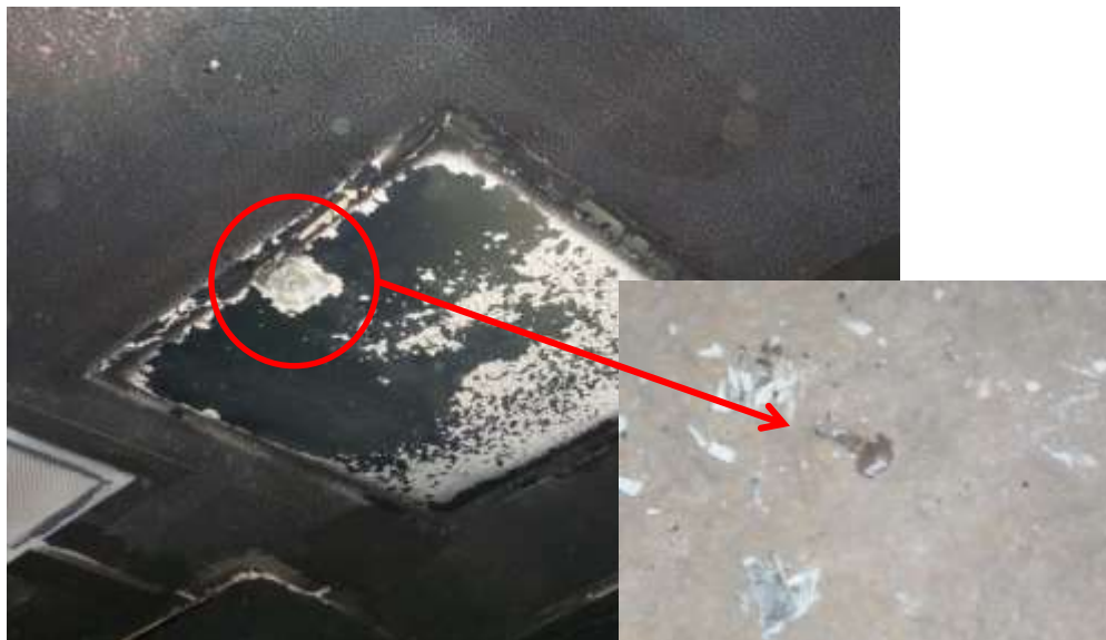
Figure 8.29. LBR access panel after LBR-2 fire test
