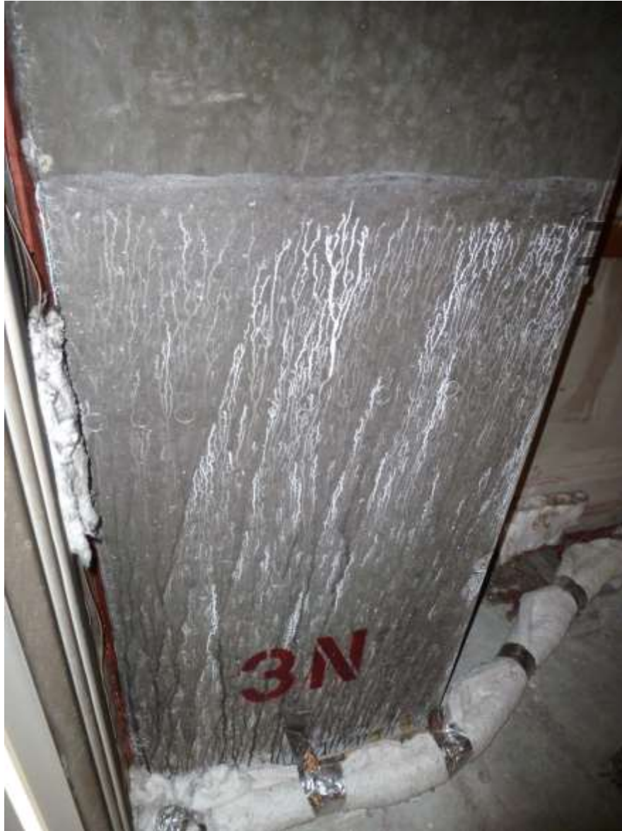
Figure 8.7. LBR northwest column after LBR-1 fire test
