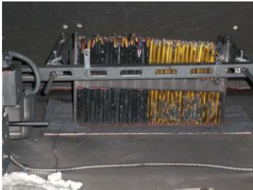
Figure 8.37. Cable tray firestop in corridor after ES fire test
