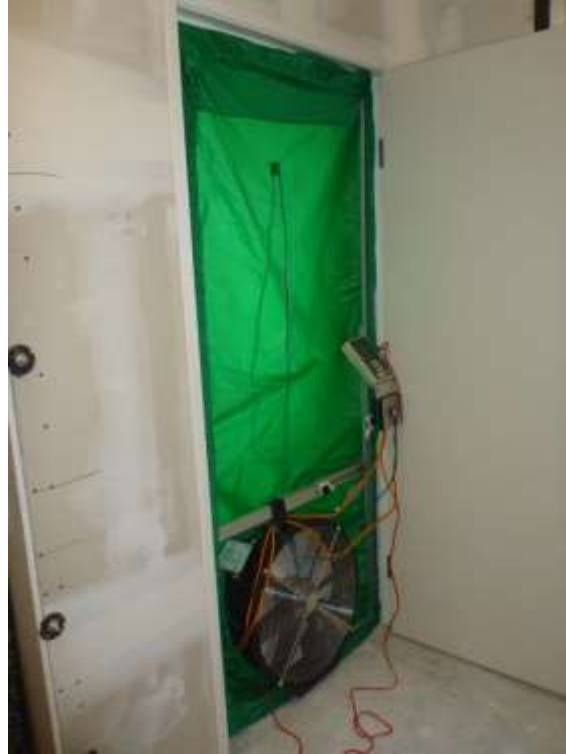
Figure 4.3. Blower door test equipment set up in door 1
