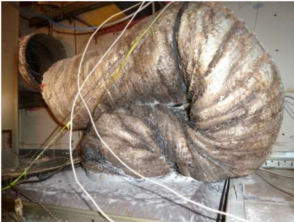
Figure 8.31. HVAC line connecting to the northwest vent of the LBR after LBR-2 fire test
