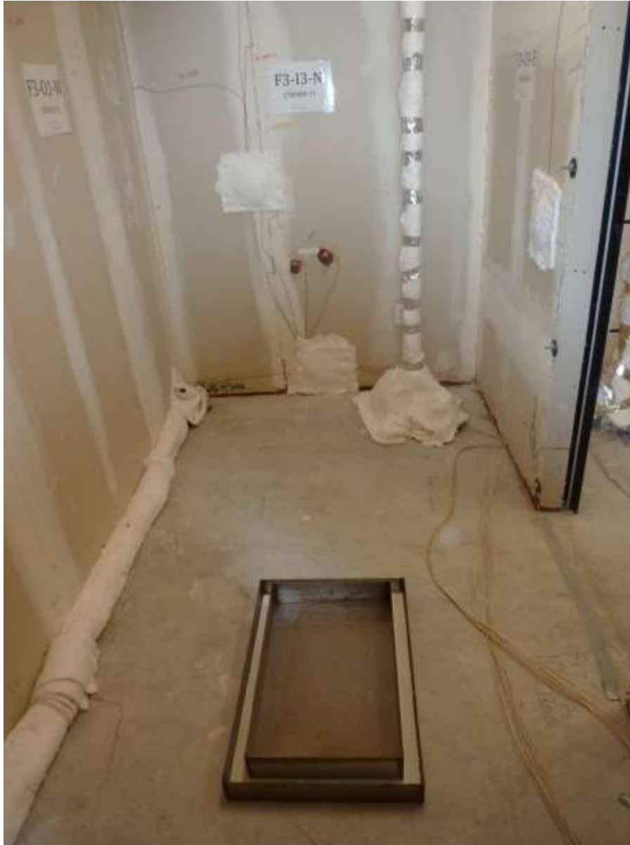
Figure 7.28. Fuel pan and thermocouple tree setup in the SBR
