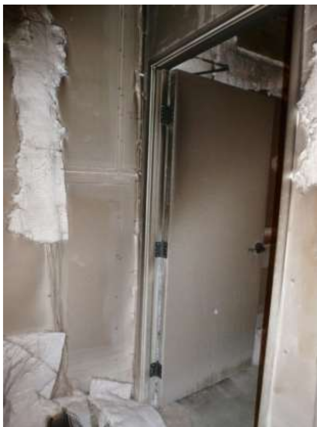
Figure 8.9. Partition wall gap after LBR-1 fire test
