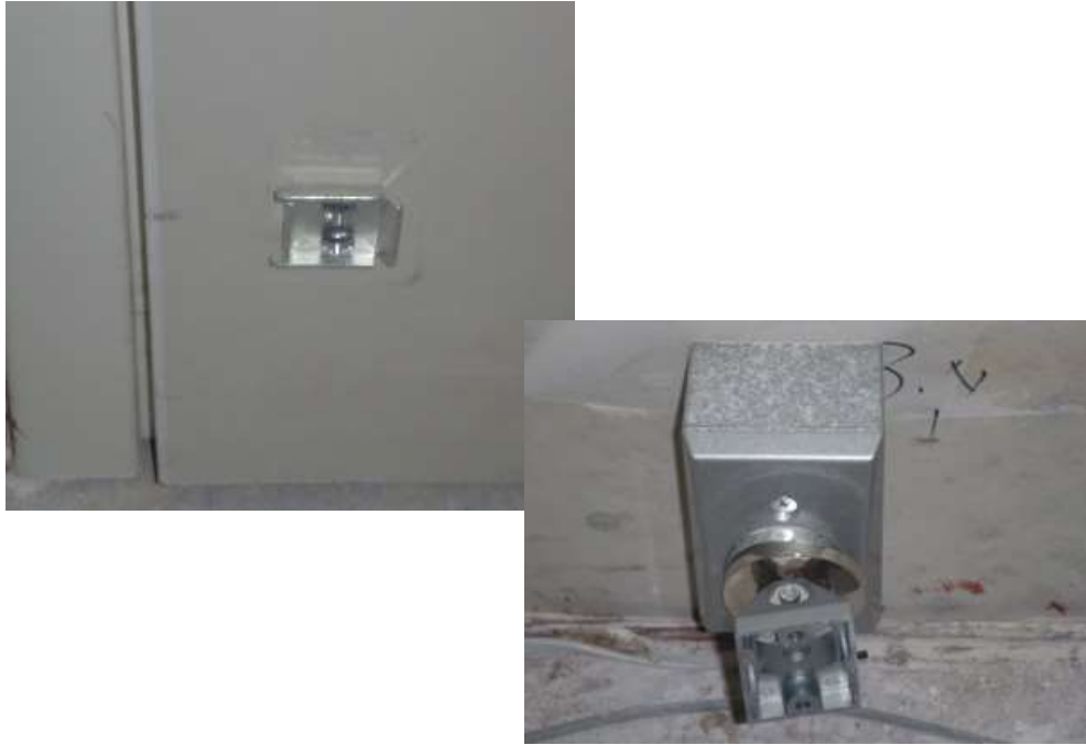
Figure 5.6. Magnetic door closer failure
