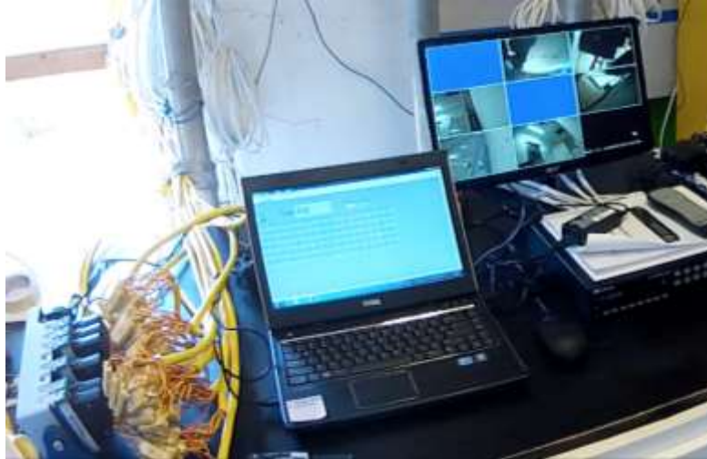
Figure 7.1. DAQ (left) and DVR (right) setup on Floor 2 for the fire tests
