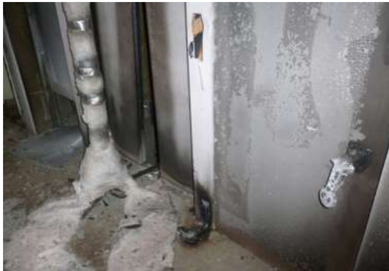
Figure 8.42. Elevator shaft wall after EL-1 fire test
