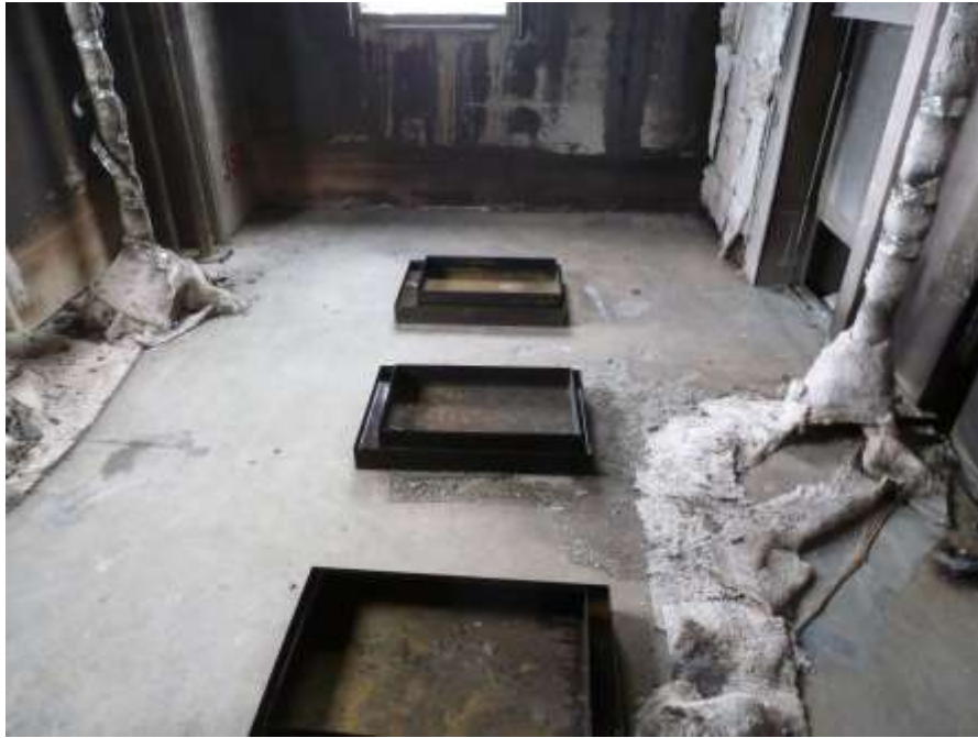
Figure 7.41. Setup of the fuel pans and thermocouple trees in the EL
