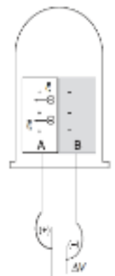
Figure 5: When we connect material A to the negative terminal of a voltage source (forward bias), current flows through the LED once the potential difference reaches a certain threshold voltage \Delta V . When this happens, the LED emits photons (represented by o).
