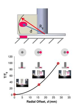
The amount of torque that the sample generates increases as the distance, **d** from the axis of rotation to the centroid of the sample increases in relation to the radius of the disc,  $\mathbf{R}_g$ . The plot above shows the increase in ratio of measured torques for a sample as it is moved from the center to the edge. This offset results in ~100-fold increase in torque relative to the centered configuration for a given angular displacement
