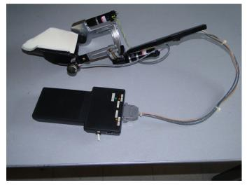
The image above shows the rehabilitation device along with a simple power pack worn on the belt. As features of the rehabilitation device, it is wearable, compact, sleek, lightweight, and not visually obtrusive.
