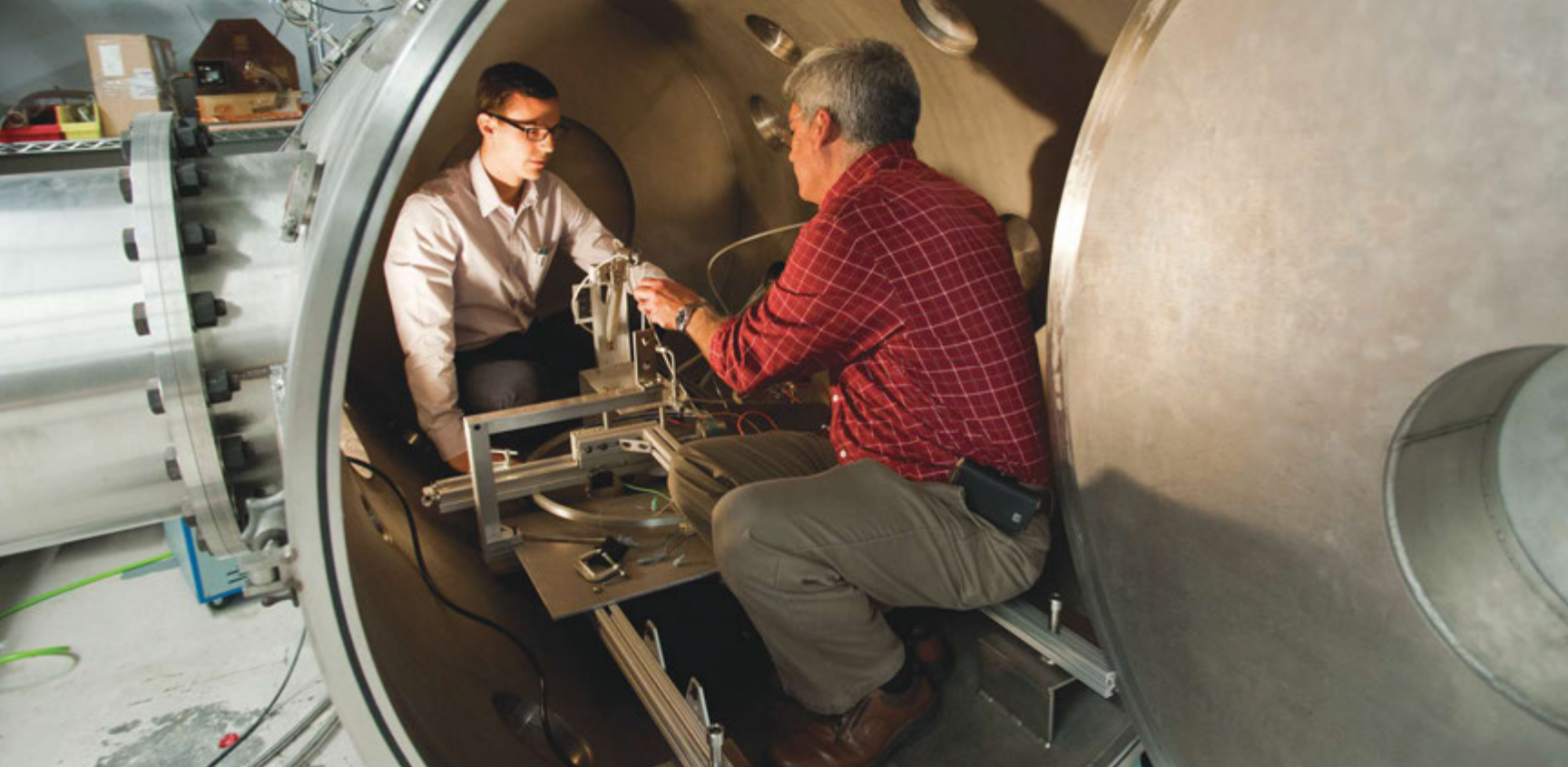
PhD student Zachary Taillefer, left, and John Blandino work inside the vacuum chamber in WPI's aerospace engineering laboratories, preparing a test of an electric thruster, like the one illustrated on page 40. They are trying to find ways to extend the life of cathodes used in spacecraft electric propulsion systems.
