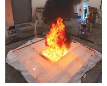
of cold and ice on oil fires. The team first observed the burning behavior of liquid fuels in cavities carved into small blocks of ice that were chilled to temperatures as low as -30 degrees Celsius in a specially designed environmental chamber.
