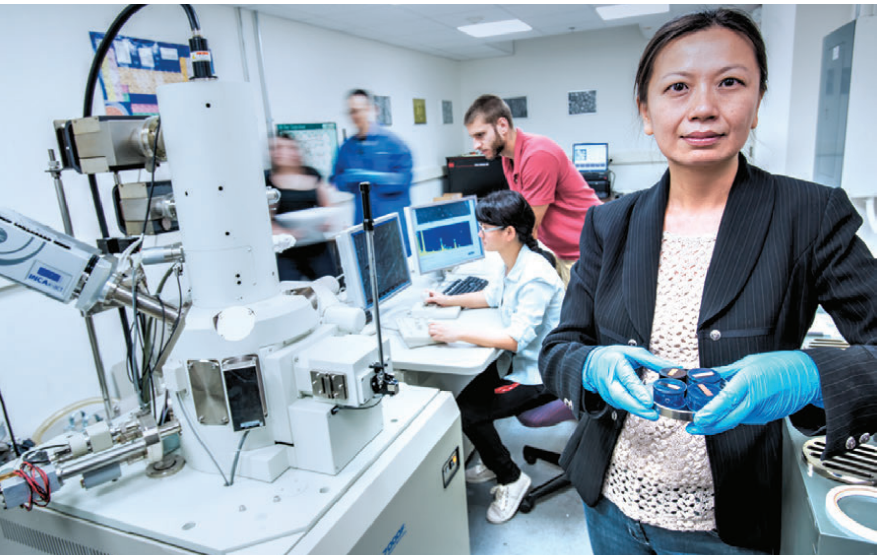
Jianyu Liang explores electrochemical finishing techniques that can reduce the vulnerability of additively manufactured parts to fatigue and cracking, and uses the scanning electron microscope to observe the effects of those methods. Behind her are, from left, PhD candidates Andelle Kudzal, Yinjie Cen, Yangzi Xu (sitting), and Ryan Mocadlo.
