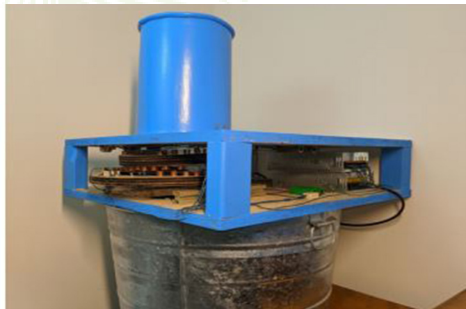
Figure E. Shred step of prototype atop basin for clean step
