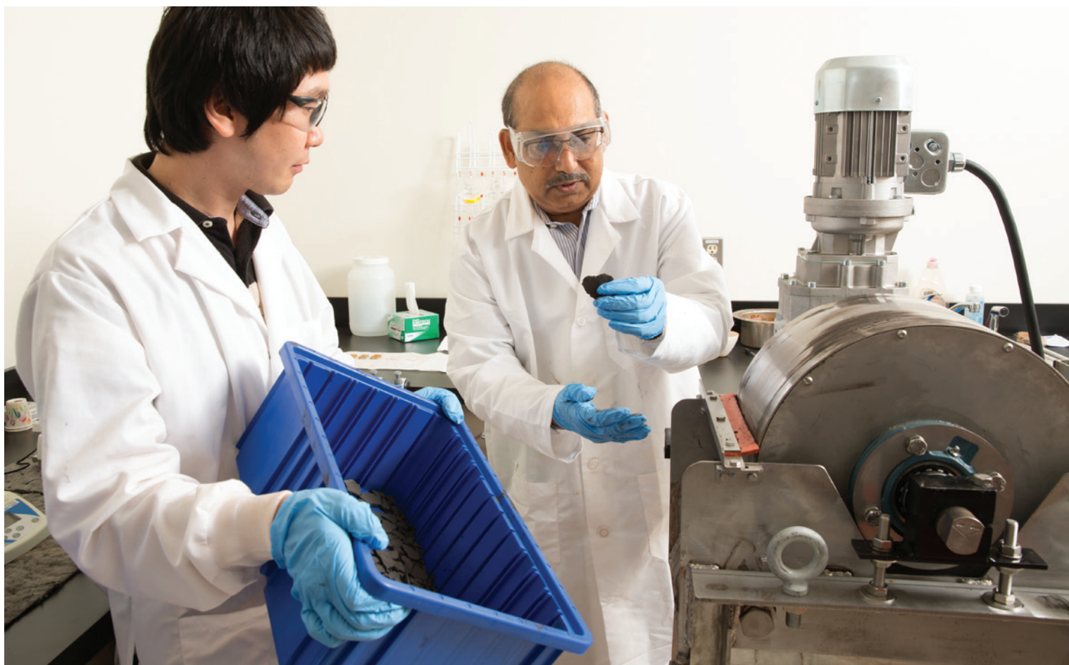
Above: Brajendra Mishra, right, and postdoctoral researcher Hyunju Lee, PhD, test technology that uses a strong magnet to recover iron oxide from treated red mud. Iron oxide, left, which makes up 60 percent of red mud, can be used in products for construction and agriculture.
