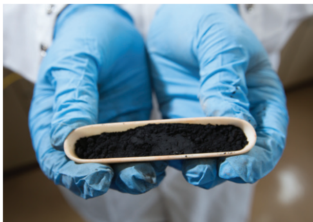
Above: Brajendra Mishra, right, and postdoctoral researcher Hyunju Lee, PhD, test technology that uses a strong magnet to recover iron oxide from treated red mud. Iron oxide, left, which makes up 60 percent of red mud, can be used in products for construction and agriculture.
