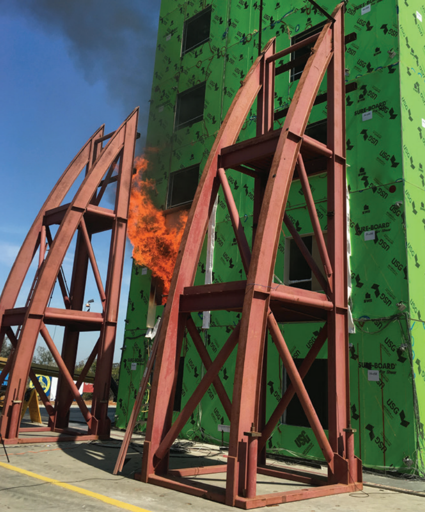
Above: A fire test under way in a cold-formed steel structure built atop the University of California San Diego's outdoor shake table. Left, Brian Meacham, at left, watches the test with Tara Hutchinson (UC San Diego) and Dan Arthur (WPI research assistant).
