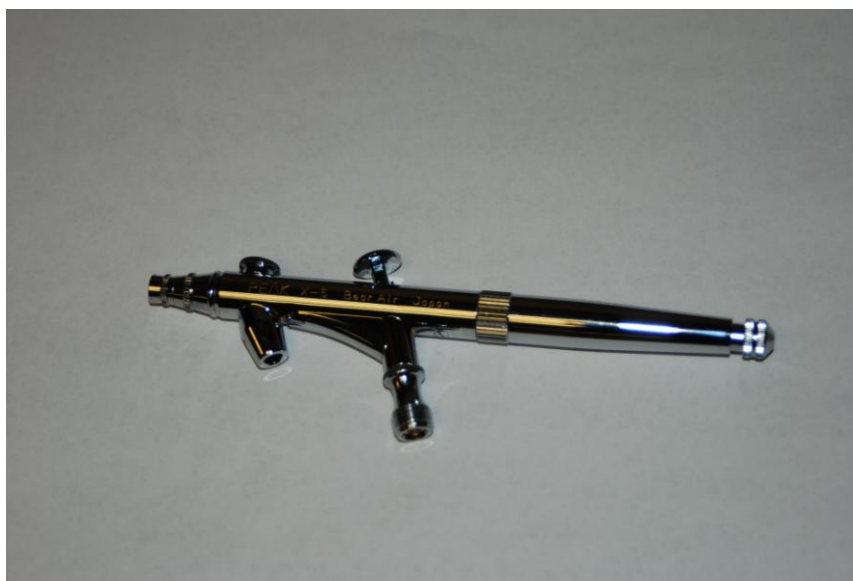
Figure 12. The Badger Professional 150 air brush gun with which the catalytic ink was applied onto the membranes.
