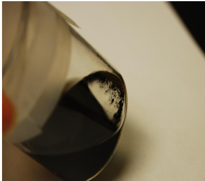
Figure 8. Solid particles form at the bottom of the catalyst ink and need to be dispersed.
