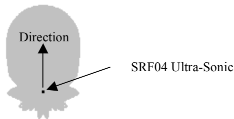
Figure 1. Beam Pattern for the Ultra-Sonic Ranger
