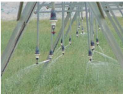
Figure 10 - Low-Pressure Center-Pivot Irrigation System 97
