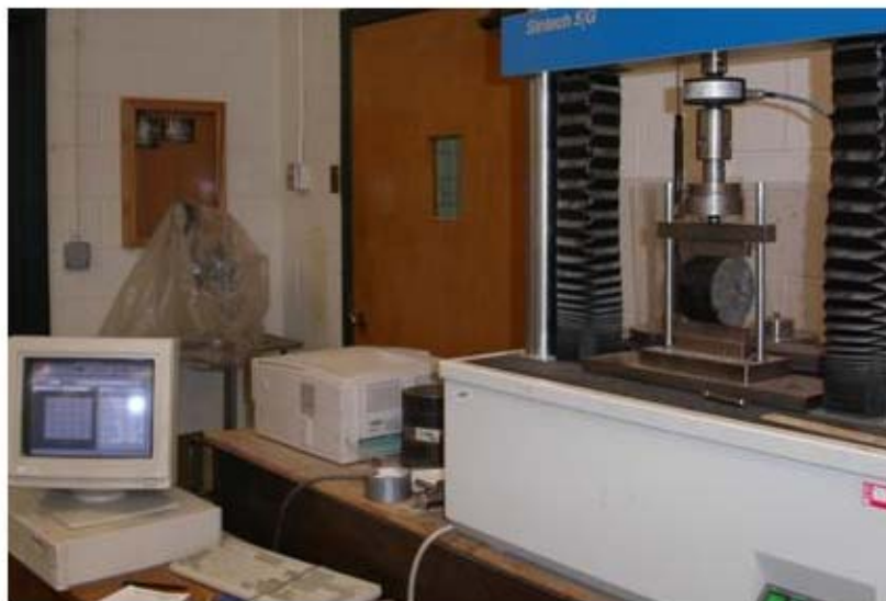
Figure 2.6. Mechanical Testing Machine by Sintech
