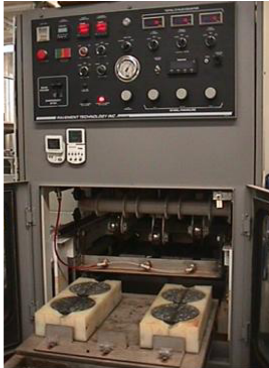
Figure 2.8. Asphalt Pavement Analyzer
