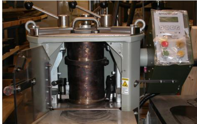
Figure 2.4. Superpave Gyratory Compactor
